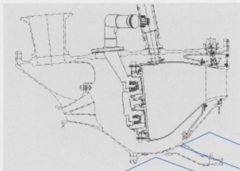
图 21 GE90 DAC TAPS 燃烧室 Fig. 21 GE90 DAC TAPS combustor
